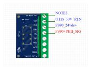
GENERIC WIRING EXAMPLES FS90 Simple V8 Use correct connections for each individual system.
