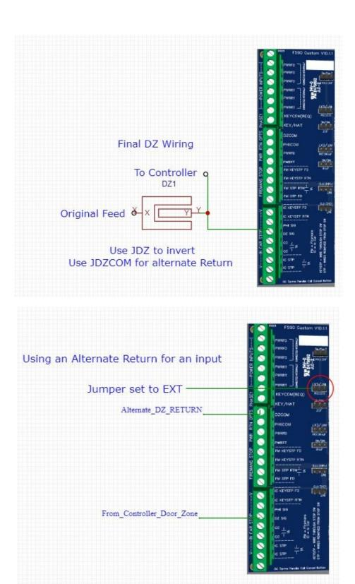
Most inputs can be totally isolated by using the INT/EXT jumper for that input. EXT connects the COM terminal for that input to the return for that input. In the above example, the DZ\_SIG input connects to one side of the DZ monitoring coil, and the other side connects to DZCOM terminal (there may be other logic in the circuit, so you may not read continuity at all times.)
