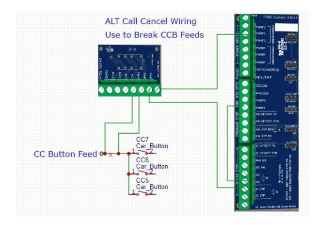
If holding the call cancel button during phase II operation interferes with PHII, you may need to use the above method of keeping the car from accepting calls.
